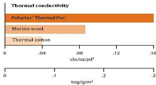
Thermal conductivity / The thermal insulation test conducted by the tester Reeves Thermal S/N 1623. Heat insulation properties are in the units clo/tog. The higher the value of clo/tog is, the better thermal properties are.
